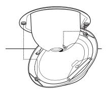
Install the lower dome. Snap the clip of the lower trim ring leash into the hole on the lip of the back box. Snap the trim ring into the plastic snap washers on the mounting screws.
